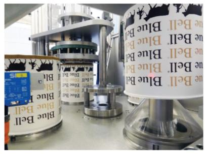
ed flexo in two colors. Like the bottom, it gets a coating of low-density polyethylene. In the drum-forming equipment at Blue Bell, the LDPE coating on the sidewall is heat-sealed to the LDPE coating on the bottom. This produces a water-tight drum without the need for gluing operations. Also notable is that this machine can be changed quickly to form drums whose fill-volumes vary.
